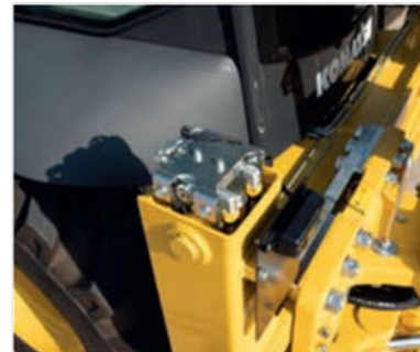
Anti-burst valves for stabilizers, boom and arm (Standard)
