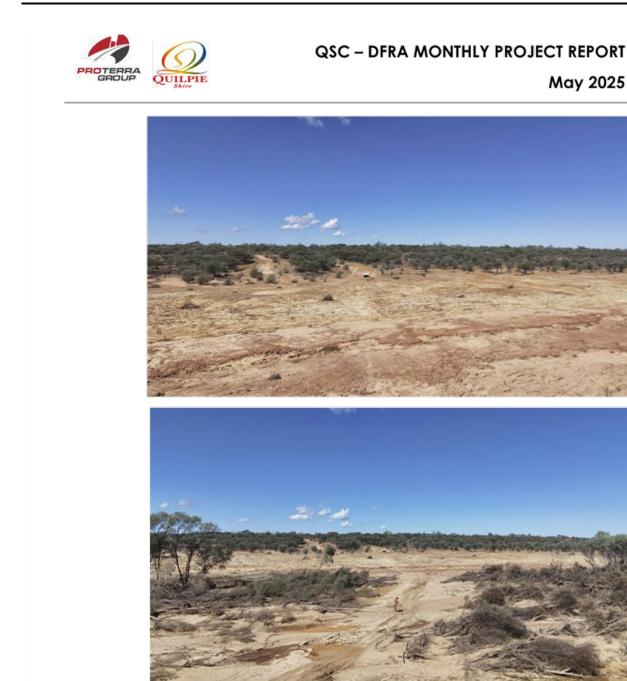
Aerial view of damaged section on Hell Hole Gorge road where overland flow has completely changed lanscape, and removed all evidence of a previous road.
