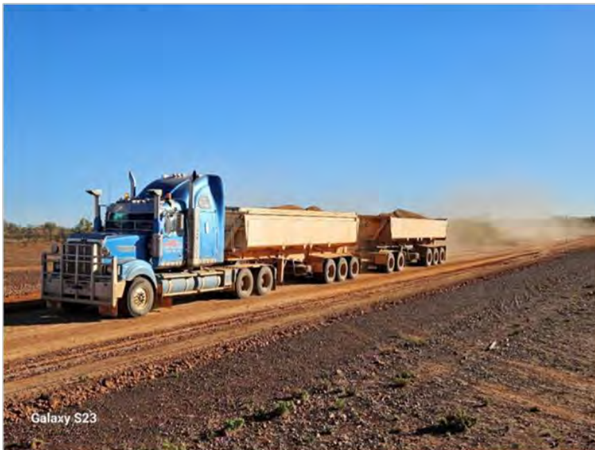
Typical equipment-Double Side Tipper used by road crews during the reconstruction of flood works in the shire to transport gravel from pits to site.
