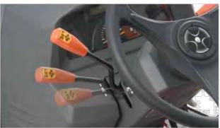
Shuttle, faster and smoother forward/reverse directional changes are easier to attain. This Carbon-Cone design makes shuttle shifting lighter and easier for instant responses, especially during front loader work.
