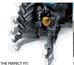
New Holland's T6000 range is designed to incorporate a fully integrated, factory fitted, front linkage and PTO. All linkage and PTO controls are positioned inside the cab for ease of operation. Purpose developed for T6000 tractors, the linkage will lift up to 3090kg. Linkage arms can be folded when not in use, or can be used to carry the new mono block front weight pack.
