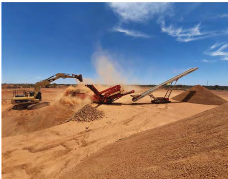
Preparation of material by screening contractor at the Congie Road pit.
