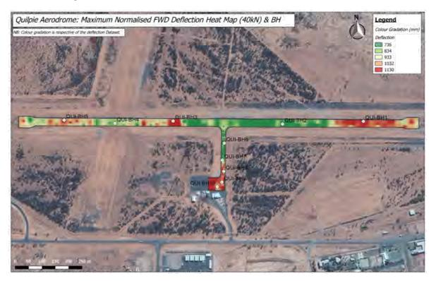
Figure 2-1 Pavement Deflection Heat Map and Borehole Locations
