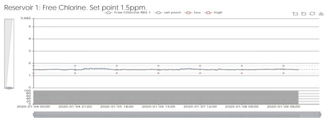
Free chlorine measurement on potable system.
