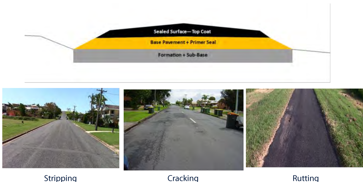
Figure 3.2.a Sealed Road Typical Cross Section and Defects
